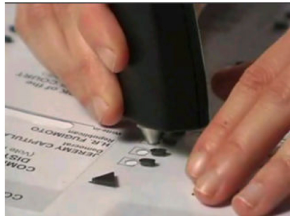
Figure 2. Light sensing verification wand.
