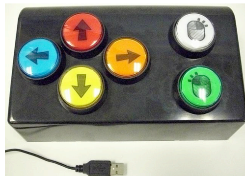
Figure 3. Large, tactile button box proposed as a possible DRE input method in future mock election studies.
